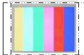
NORMAL/PS mode crops the left and right side of image to eliminate the black stripes. The image will remain the original ratio
