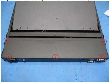
**Step 2:** Remove the bearing plate, and then remove the 2 screws under the place. (Both sides)
