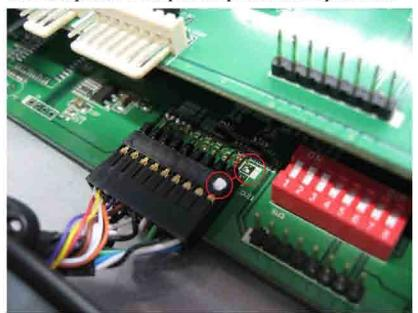
NOTE: When connect back the cable, please make sure the "white dot" is facing up to match the right pin-out.
